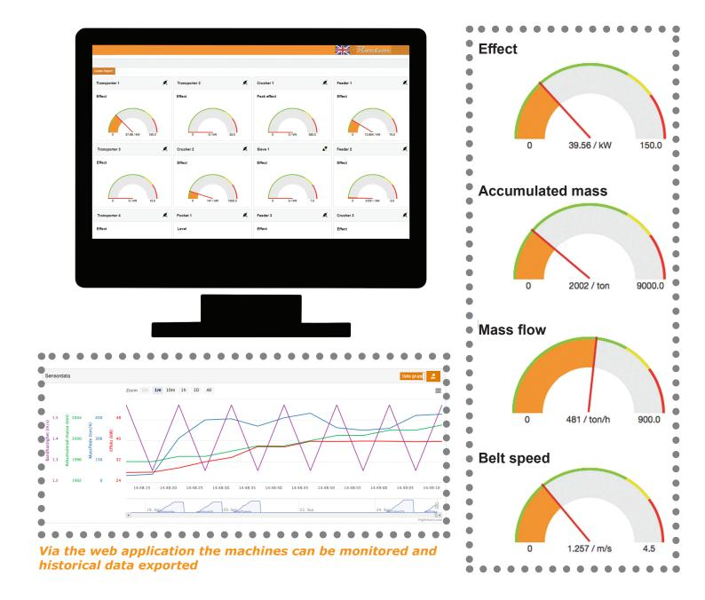
Roctim's cloud solution works very well together with our CCU (Crusher Control Unit) Base, which offers an advanced protection agains overload and maximizes the production.
